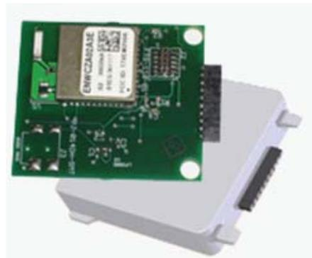
The user-replaceable U-SNAP module shown here measures only 1.5 inches (3.8 cm) square. The plastic enclosure protects the circuitry while providing convenient access from the exterior of the device. A HAN Device Portal designed to use plug-in U-SNAP modules offers the consumer greater flexibility while offering the utility a future-proof approach to the HAN.
